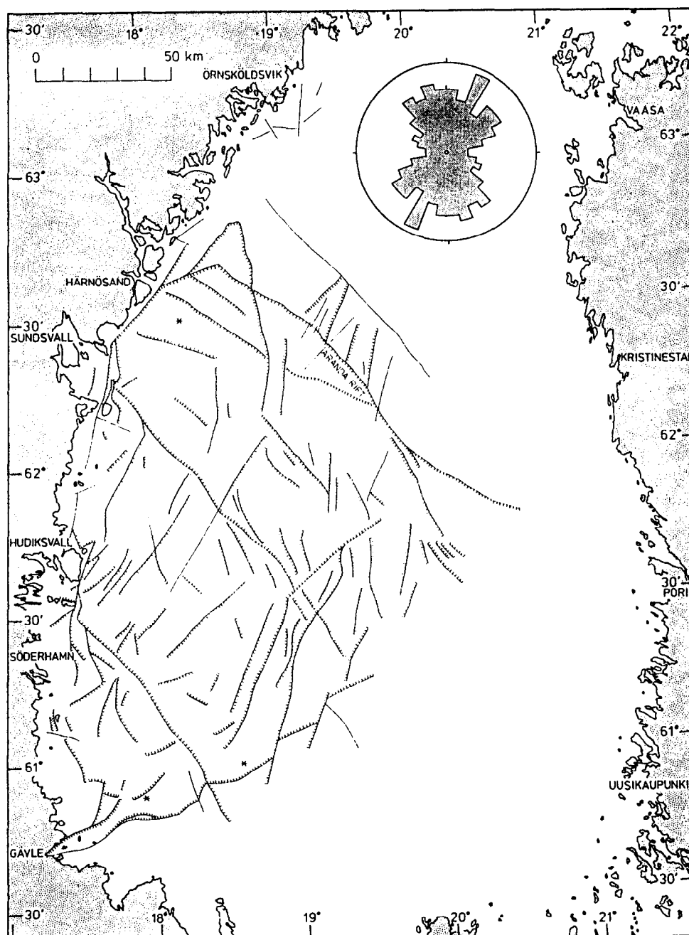
Fig. 5. Fault trace map of the Bothnian Sea, derived from bathymetric maps and shallow seismic reflection and refraction profiles (taken from Axberg, 1980). The rose diagram shows the distribution of fault strikes.
